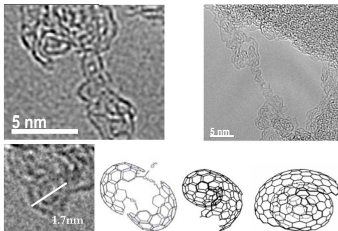
**Fig. 4.** Small transitional objects between molecules and solid soot grains observed in HT condensation experiments.
