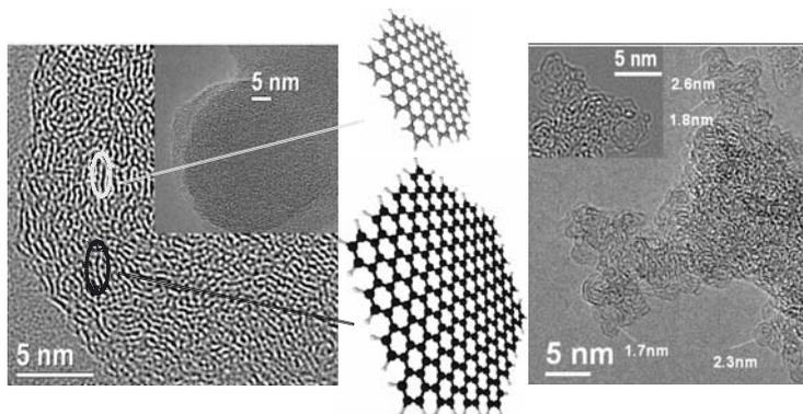
**Fig. 2.** HRTEM micrograph of a grain formed in a LT (left) condensation process. The average length of graphene layers is around 2 nm comparable to PAHs with masses of around 1300 u (smaller PAH molecule). The largest layers have a size of 3 nm which corresponds to PAHs of about 2700 u (large molecule). The HT condensed grains in the right panel are built of fullerene fragments or bucky onions with nested fullerene cages.
