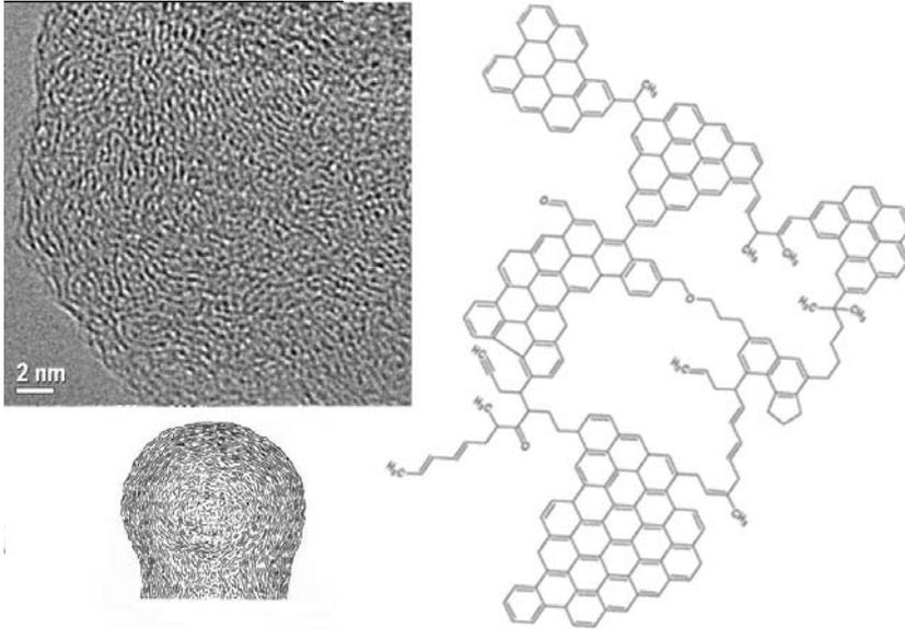
**Fig. 1.** HRTEM image of a gas-phase condensed particle having a paracrystalline structure. The chemical formula (right) shows one possible amorphous carbon structure which can be considered as a paracrystalline graphene layers.
