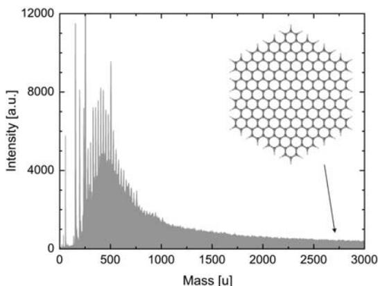
**Fig. 3.** MALDI TOF spectrum of a LT soot sample showing PAHs with masses up to 3000 u. To exemplify a PAH molecule with comparable mass, a molecule comprising 91 condensed rings is presented.
